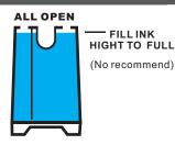
When you want to filling ink, firstly, please pull out the rubber plugs from the fill-hole of the ink tank; use a common syringe to fill ink (please see the step as picture 2); and then, pull out rubber plugs from the CIS cartridge and use a syringe to draw air, pull the syringe position for air-removing (please see the step as picture 3), then the ink will flow into the ink cartridges from the tanks automatically. After filled, you need to stuff all holes with the rubber plugs.
