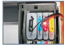
Open cover for Inkjet cartridges. Remove the original cartridges. Insert our no-sponge cartridge into printer carefully.
