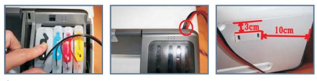
Slightly press every cartridge to check all the cartridges are in the correct position. Please be careful with the tubes which go out from Cartridge Carrier. Then stick the Support Arm on the position which shown in the third picture.
