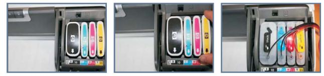
Open cover for Inkjet cartridges. Remove the original cartridges. Insert our no-sponge cartridge into printer carefully.
