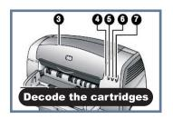
When the printer says change the cartridges, need to decode the cartridges. Just press the button 6 (restore key) till the light does not flash, then it is decoded.
