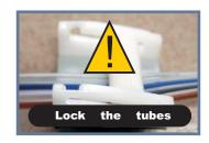
When you need move the ink tanks, or move the cartridges, please lock the tubes with the tube lock
