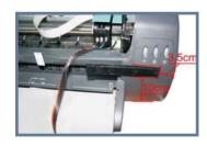
We have installed the support arm in the cartridges.
