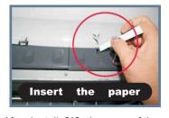
After install CIS, the cover of the printer can not be closed well , just insert the paper to the hole as picture shows.
