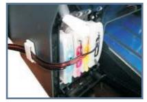
Use paper make taper style and Insert the paper into the printer hole. Then cartridge-cover can be recognized cover well. Finished.
