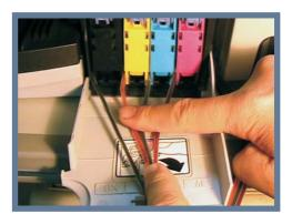
1 Pipelines must go through the gaps on the bottom
