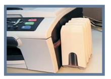
1 Pipelines must go through the gaps on the bottom
