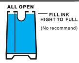
When you want to filling ink, firstly, please pull out the rubber plugs from the fill-hole of the ink tank; use a common syringe to fill ink (please see the step as picture 2); and then, pull out rubber plugs from the CIS cartridge and use a syringe to draw air, pull the syringe position for air-removing (please see the step as picture 3), then the ink will flow into the ink cartridges from the tanks automatically. After filled, you need to stuff all holes with the rubber plugs.
