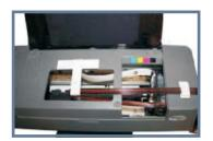
**5** Clip the tube Move the carriage to the rightmost and make sure that the tube can be straight. Installation is finished.
