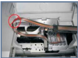
Tube excessive long
