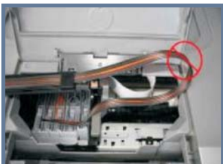
Tube excessive long
