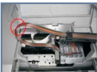
Tube excessive long
