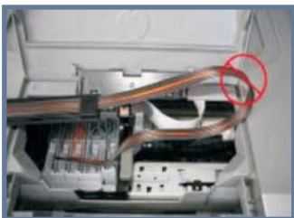
Tube excessive long
