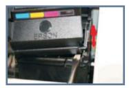
2 Open the carriage cover to certain angle (about 60 degree). Then use a screwdriver to insert into the joint as the picture shows.
