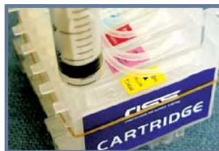
NEED REMOVE AIR WHEN FILL INK INTO EMPTY INK SYSTEM AT 1ST TIME
