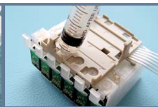
NEED REMOVE AIR WHEN FILL INK INTO EMPTY INK SYSTEM AT 1ST TIME
