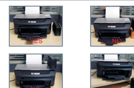
Keep the ink tanks and printer in the same level. Do not place the tanks higher or lower than their printer
