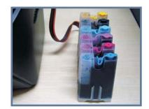
The CIS are used with the air balance design. After filling ink or moving tanks, you should do these like the above pictures. Inverse the tanks, let most of ink flow into big sides.
