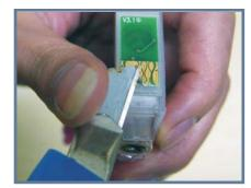
Some chip parts might be pressed to a lower position, you need to cut the higher mast by a knife.
