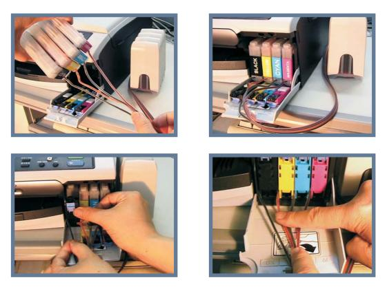
I Pipelines must go through the gaps on the bottom
