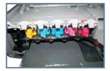
Open the top cover, take out the original cartridges. Before you install the CIS cartridges, please make clear the chip position and make sure that each color cartridge will
