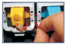
Close the top cover. Thread the tube through the cartridges clip. Tear the tubes among the cartridges about 2 cm it will be easier to install the color cartridges. Make sure the tube line between each two clips are not folded. Pull the tube slightly to see if it is installed well.
